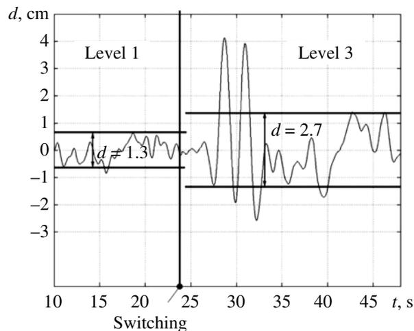
Fig. 6. Change in the levels of pilot ratings in the event of a failure.
