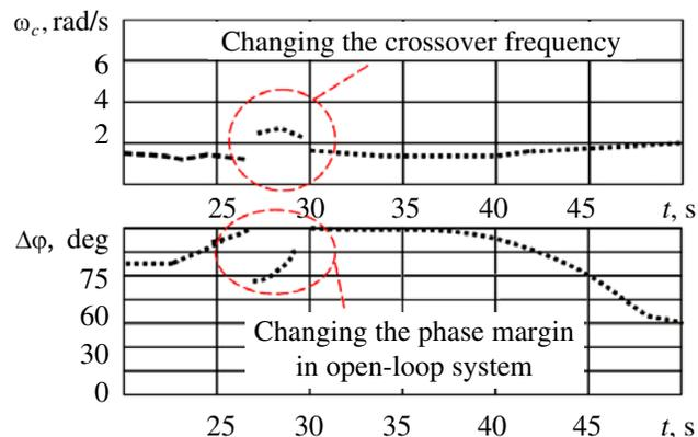
Fig. 7. Change in the characteristics of the open-loop pilot–aircraft system in the event of a failure.
