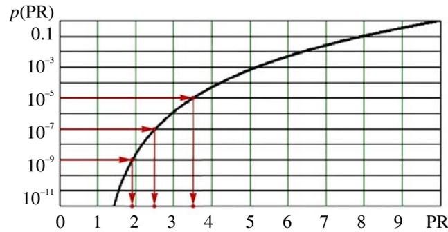
Fig. 5. The dependence of the probability of a flight accident on the average rating of flying qualities.
