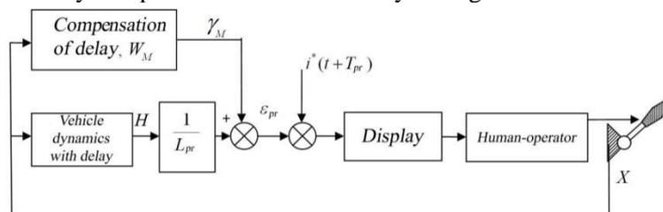
**Figure 2.** Compensation of time delay
