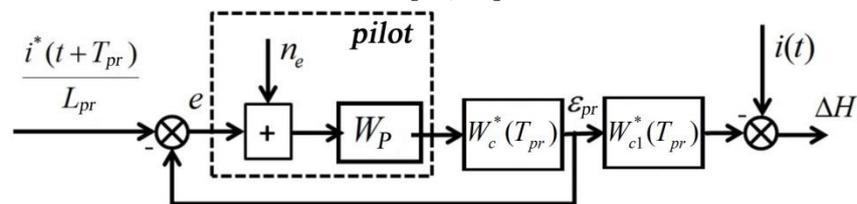
**Figure 1.** Pilot-aircraft system with predictive display
