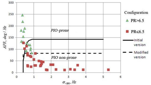
**Fig. 4 Phase rate criterion.**
