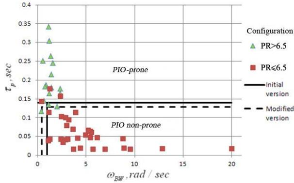
**Fig. 3 The  $\omega_{BW} - \tau_p$  criterion to evaluate the PIO.**
