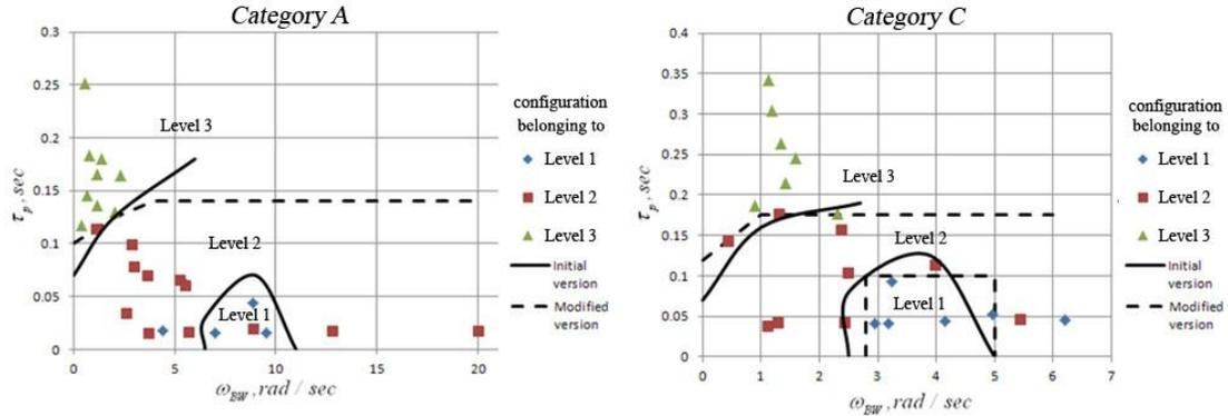
**Fig. 2 Bandwidth criterion for the different flight evaluation categories.**
