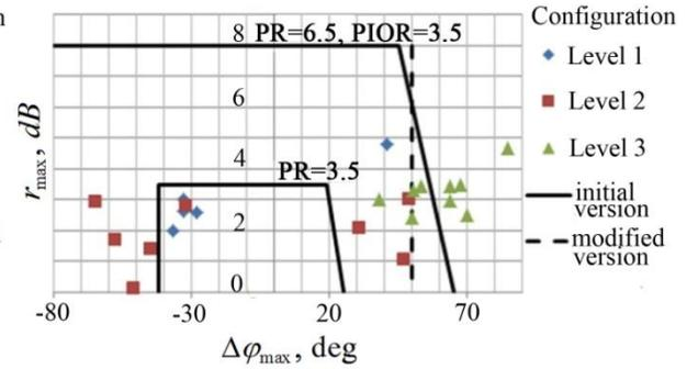
**Fig. 7 Modified MAI criterion ( $r$  and  $\Delta\varphi$ ) found from the optimal pilot model.**
