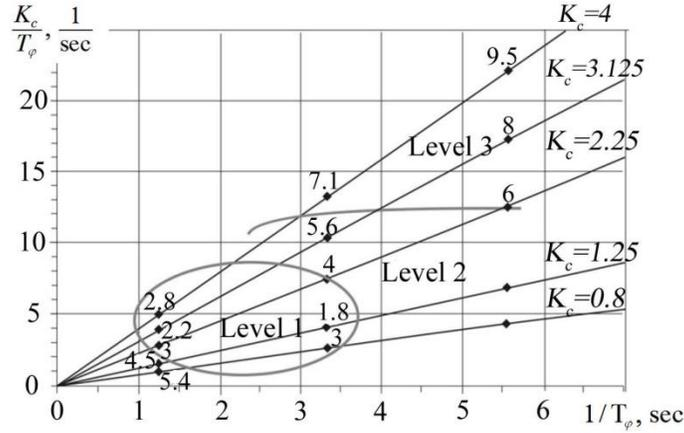
**Fig. 15 FQ requirements for roll control tasks.**
