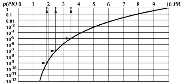
**Fig. 20 Estimation for the probability of an accident.**
