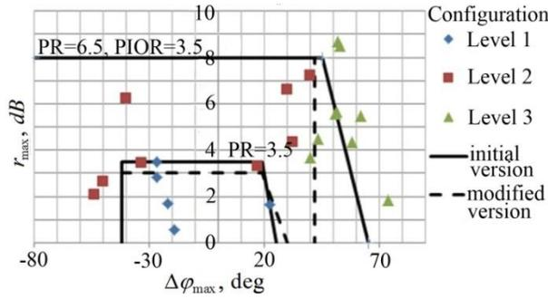
**Fig. 6 Modified MAI criterion ( $r$  and  $\Delta\varphi$ ) with boundaries found from experiments.**
